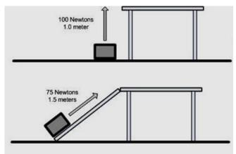
In this example, it takes 100 newtons of force and 100 Nm of work to lift the box, and 75 newtons of force and 112.5 Nm of work to push the box up the ramp. If the person moving the box has only 80 newtons of strength, he will not be able to lift the box, but will be able to push the box up the ramp. The trade-off is that more work is done to push the box up the ramp, because some work is lost to friction on the ramp.
