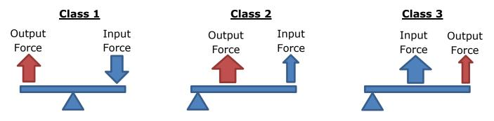
In each class of lever, the difference between the lengths of the input and output arms determines the mechanical advantage. The further away that the input force is from the fulcrum, as compared to the output force, the greater the magnification of force and mechanical advantage.
