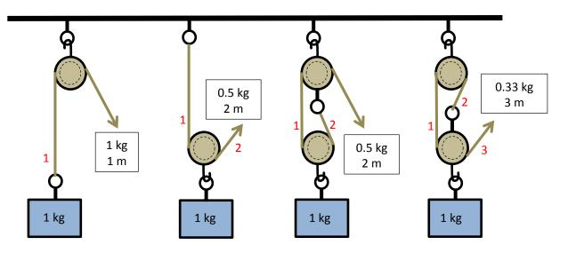
Notice that in each pulley arrangement, the total work performed is the same, about 1 joule (N•m), even though the amount of input force and input distance (shown in the box next to the input force arrow) varies. To find the **ideal mechanical advantage** (the magnification factor of the force, disregarding friction) of a pulley, simply count the number of ropes <u>leading away</u> from the weight being lifted (the small red numbers next to the ropes show this count).
